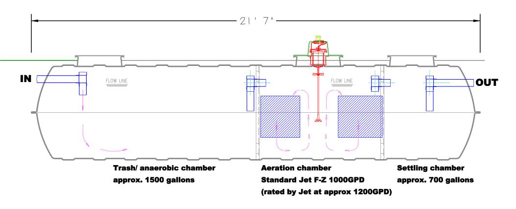
Fibre-Zone 'super septic' system 3000 USG
